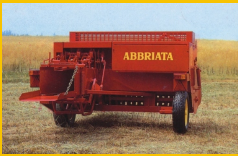
Vista posteriore con ruota montata a tergo raccogliitore Rear view with the side pick-up wheel mounted behind
